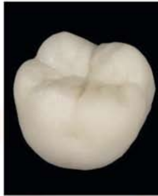
Ceramic crown after press-molding
