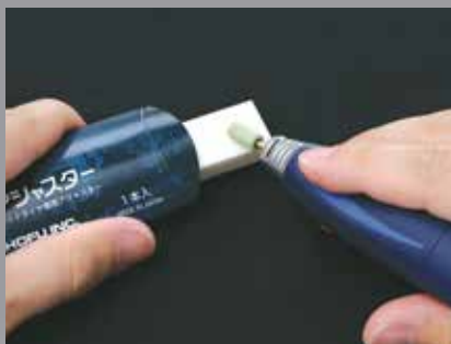
Press Dura-Green DIA against the Shofu Adjuster while rotating the abrasive
