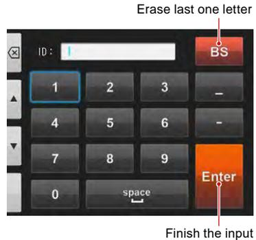
The keypad shows an 'ID:' field with a cursor. A red arrow points to the 'BS' key with the label 'Erase last one letter'. Another red arrow points to the 'Enter' key with the label 'Finish the input'.
