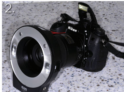
2. Newer SLR systems deal with the weight and ergonomic issues by using a shorter, 85 mm lens and wireless flash.
